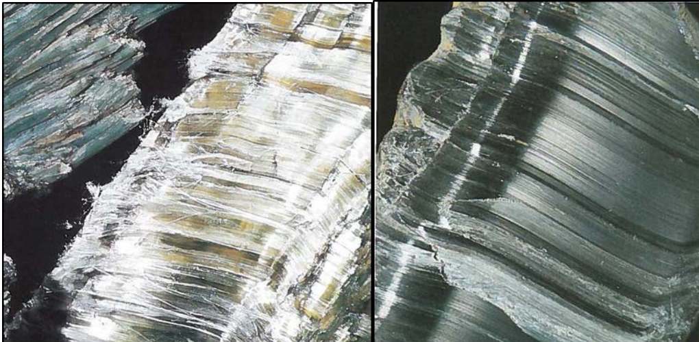
Figure 3: Illustrations of chrysotile/white asbestos (left) and crocidolite/blue asbestos (right) (From: Minerals of the World, by Rudolf Dud'A & Lubos Reijl)
